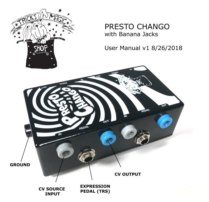
The Presto Chango is a passive adapter box that provides the use of up to 4 standard expression pedals, like the Moog EP2 and EP3, with banana jack format modular synths. The Presto Chango has been tested to work with Moog EP2 and Moog EP3 Pedals, which have TRS audio connectors. Others with a TRS connector may work, but have not been tested. Expression pedals with only a TS style connector will not work with the Presto Chango.
