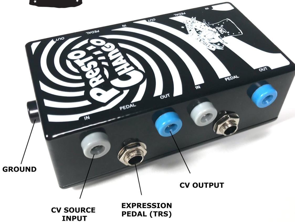
The Presto Chango is a passive adapter box that provides the use of up to 4 standard expression pedals, like the Moog EP2 and EP3, with banana jack format modular synths. The Presto Chango has been tested to work with Moog EP2 and Moog EP3 Pedals, which have TRS audio connectors. Others with a TRS connector may work, but have not been tested. Expression pedals with only a TS style connector will not work with the Presto Chango.
