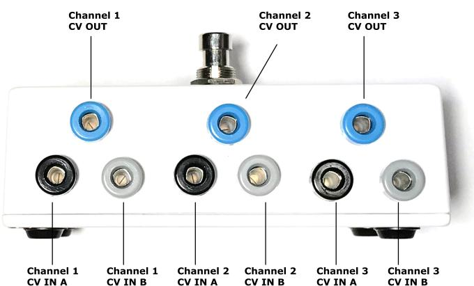
The Sleight of Hand with Banana Jacks is a passive, three-channel, CV (control voltage) signal footswitch for modular/semi-modular synthesizers. Upon the click of the footswitch, up to three CV source signals switch between their respective A and B inputs to their correlating outputs. All three channels switch simultaneously. Clearly, you can just use a single channel as well by simply using, for example, only the Channel 1 CV A & B Inputs and the Channel 1 CV Output.
